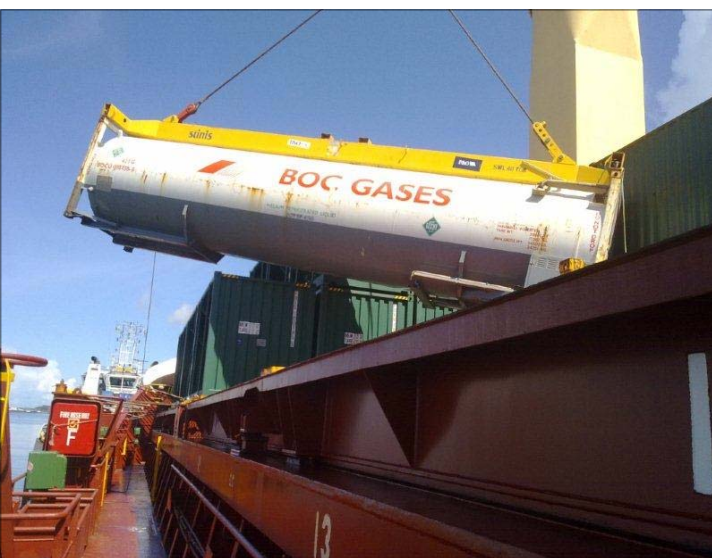
Ship's crane in Darwin uncontrollably booms up with 40ft hazardous box
