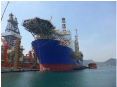
When complete, she will then be towed into the Field and positioned approximately 3.5 kilometres away from the Ichthys Explorer–central processing facility. The facility's turret will be hooked up to 21 mooring chains, the risers and then umbilicals will be connected and commissioned. The production phase that will start at the end of this year.
