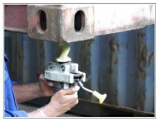
The RAM PinSmart automates the task thereby reducing the need for workers to be in these hazardous situations. RAM has utilised its 30 years of experience in designing spreaders operating in onerous conditions to now produce a machine that automates the task of handling twistlocks.
