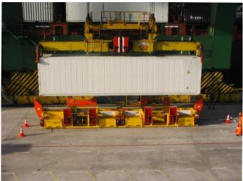
The RAM PinSmart machine is lifted and moved by a standard telescopic spreader at the 20ft position and can be quickly and easily transferred from bay to bay by a ship to shore crane or straddle carrier.
